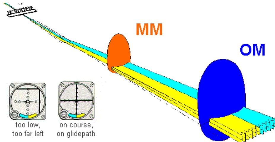
Above is a three-dimensional depiction of the Instrument Landing System. Localizer antennas shown at far end of runway.
