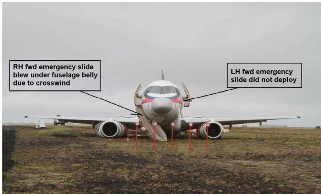
Figure 6: Forward RH emergency escape slide unusable
