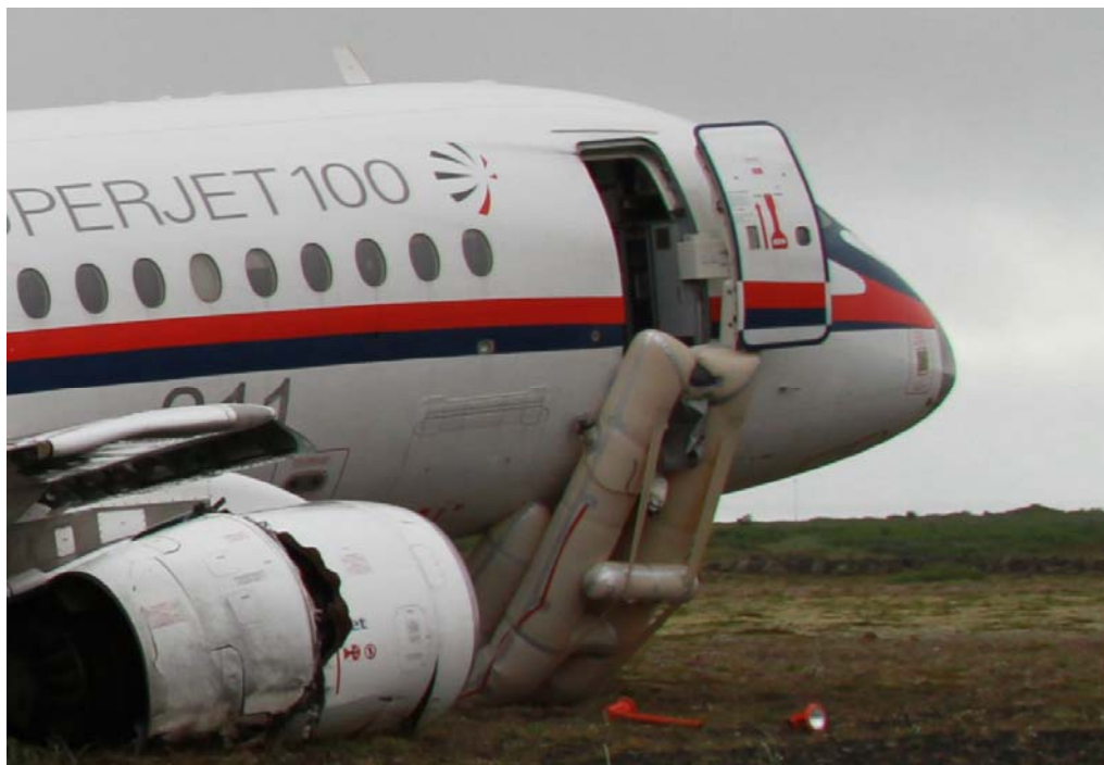
Figure 16: Forward right cabin door slide unusable
