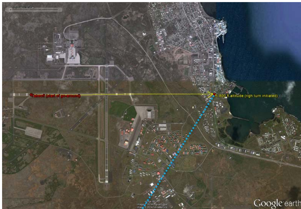
Figure 17: Calculated track from takeoff to 800 feet altitude under test condition
