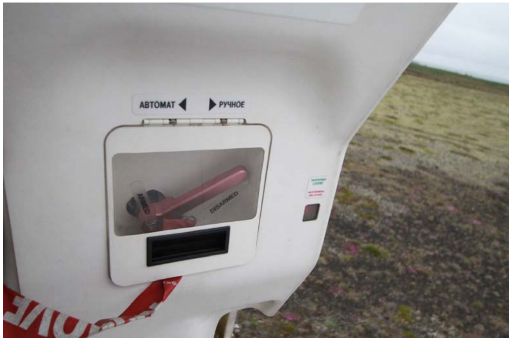
Figure 15: Forward left cabin door slide was not armed
