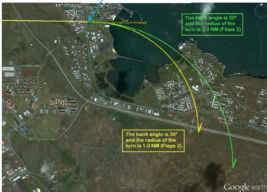
Figure 18: Turn based on right turn at 800 feet altitude for 20° / 30° bank angle
