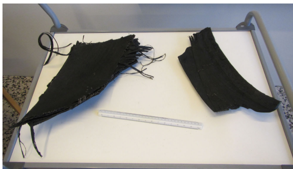
Figure 7: Tire rubber debris found at Keflavik Airport after the takeoff
