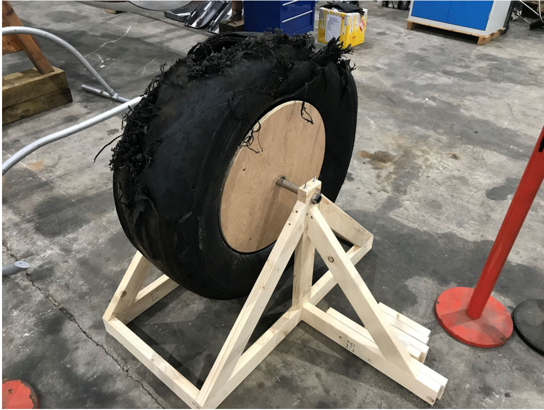
Figure 15: Tire and tire debris reassembled in a jig
