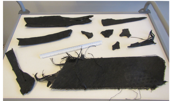
Figure 7: Tire rubber debris found at Keflavik Airport after the takeoff
