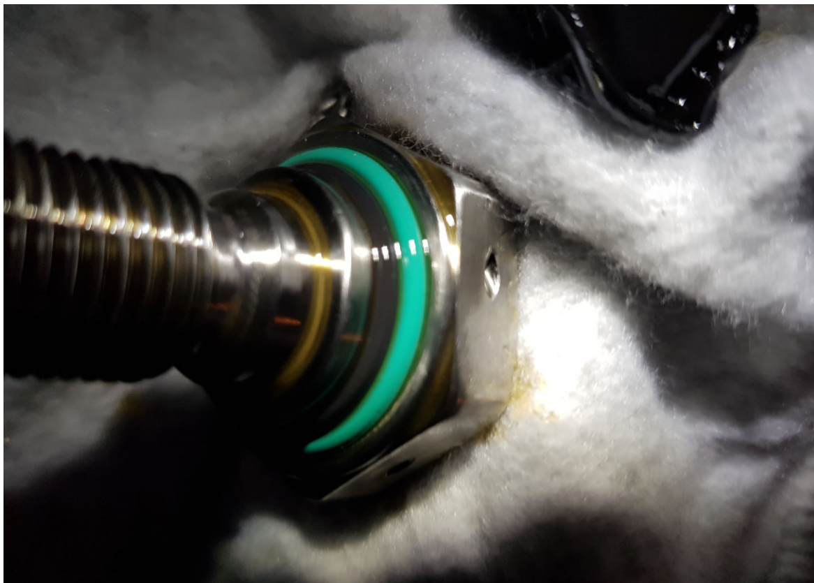
Figure 17: Black O-ring (50) nesting against green Back-up Seal (80)
