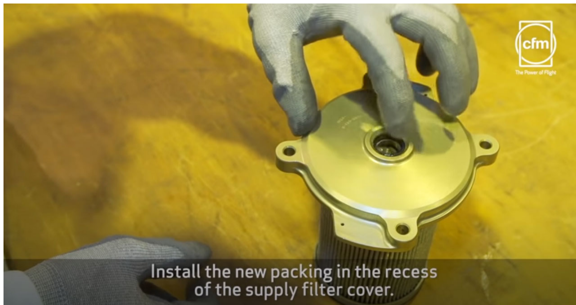
Figure 15: Install the black O-ring (50) into the filter cover (40) recess
