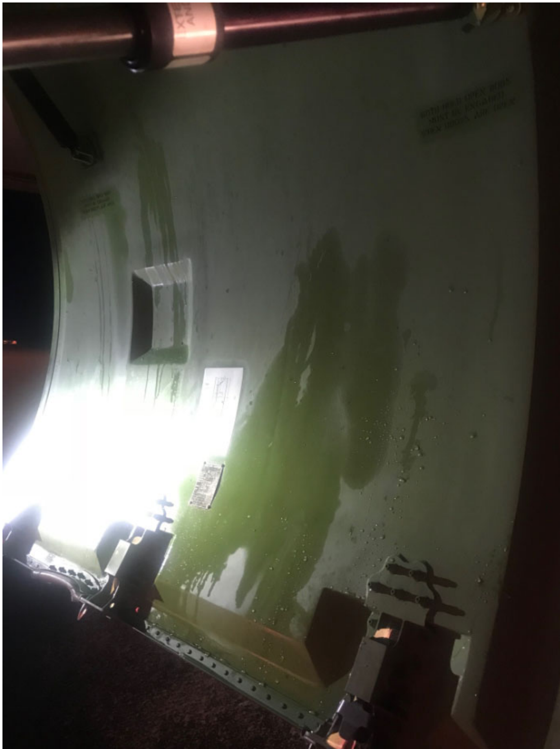
Figure 4: Engine no. 1 - The inside of the cowling was wet with oil
