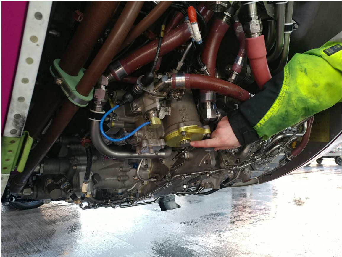
Figure 3: Engine no. 2 - Leaking oil drain plug on oil supply filter
