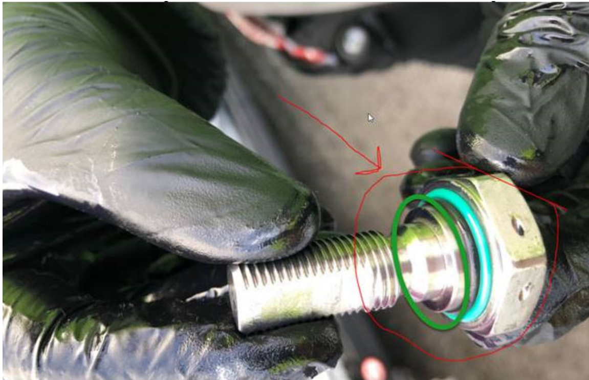
Figure 18: Correct location of O-ring (50) shown with the dark green circle
