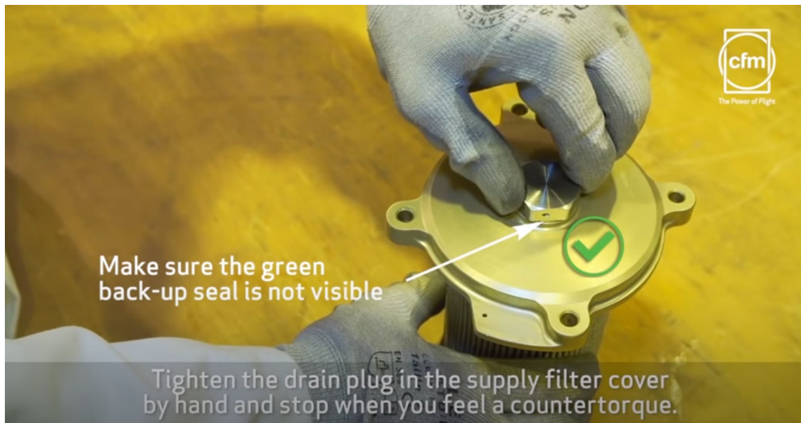
Figure 16: Fasten the drain plug (60) through the filter cover (40) and into the filter (20)
