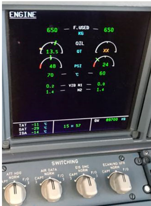
Figure 1: Photo of the ECAM after the “XX” appeared
