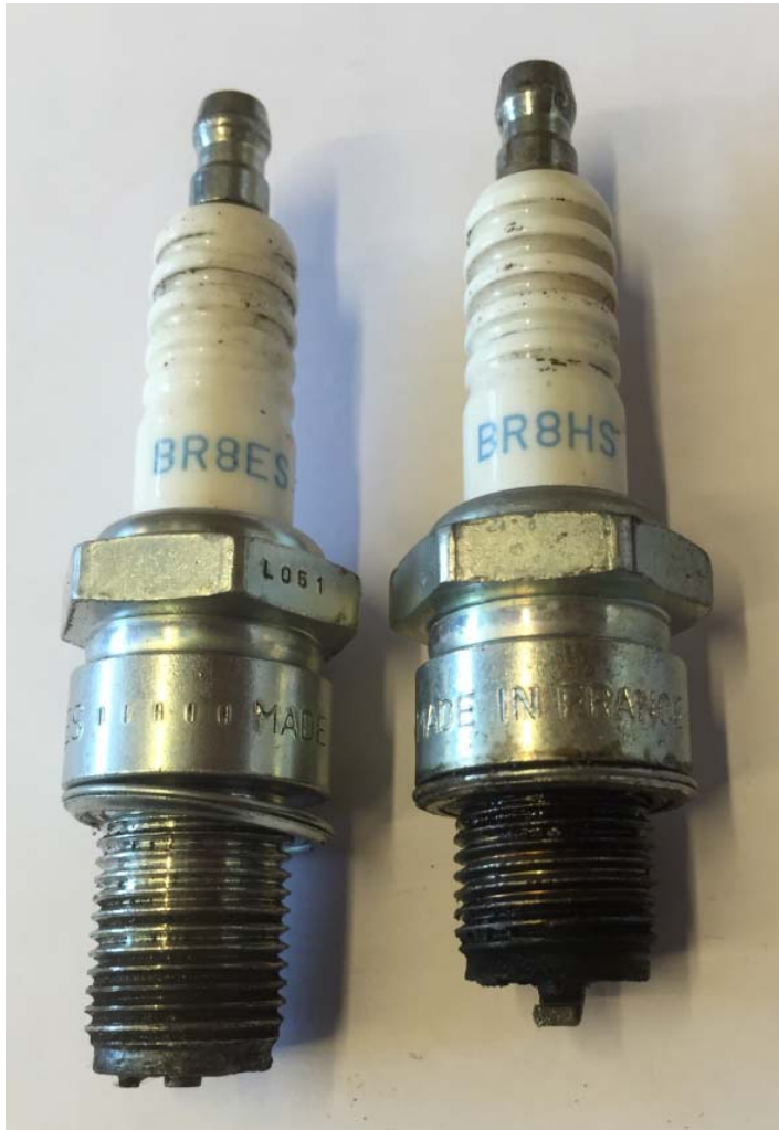
Figure 4: Installed BR 8 ES spark plug on LH side / Removed BR 8 HS spark plug on RH side
