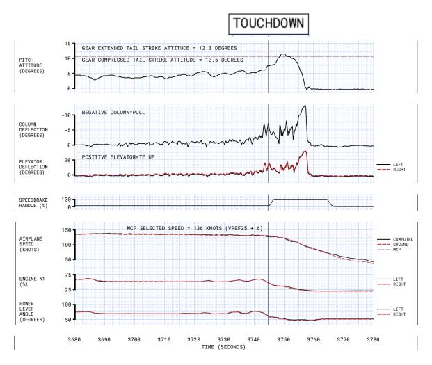
In the FCTM<sup>7</sup> it is also discussed that to avoid a tailstrike, the pilot needs to ensure that the pitch attitude does not increase after touchdown.
